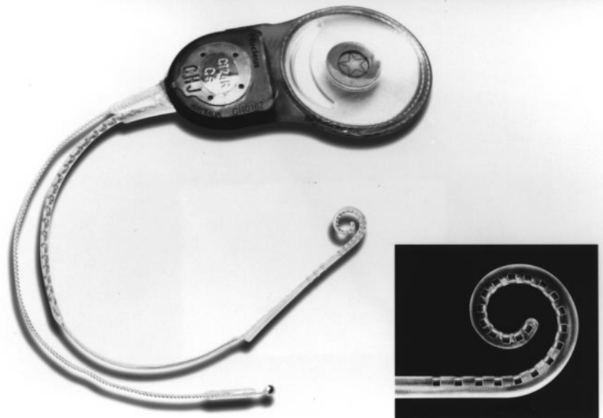
FIGURE 23–1. New electrode design that hugs the modioli after the insertion stylus is withdrawn. Courtesy of Cochlear Ltd.
