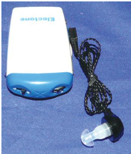
Fig. 1.18: Body level hearing aid
