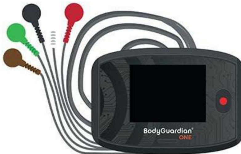
FIGURE 13.12. Example of intermittent patient- or event-activated recorder: BodyGuardian One Preventice Solutions, Inc. (BodyGuardian is a registered trademark of Preventice Solutions, Inc.)
