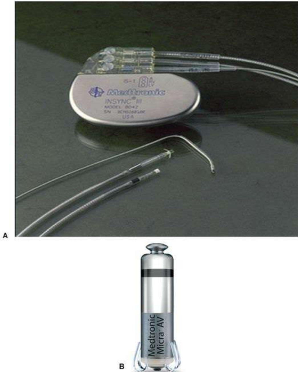
FIGURE 21.1. A. Biventricular pacemaker with three leads: top lead, coronary sinus (left-ventricular) pacing lead; middle lead, right-ventricular pacing lead; and bottom lead, active fixation pacing lead for the right atrium. B. Leadless pacemaker that incorporate the pulse generator and pacing electrodes into a single miniature unit – Micra AV Model MC1AVR1. (© 2020 Medtronic.)
