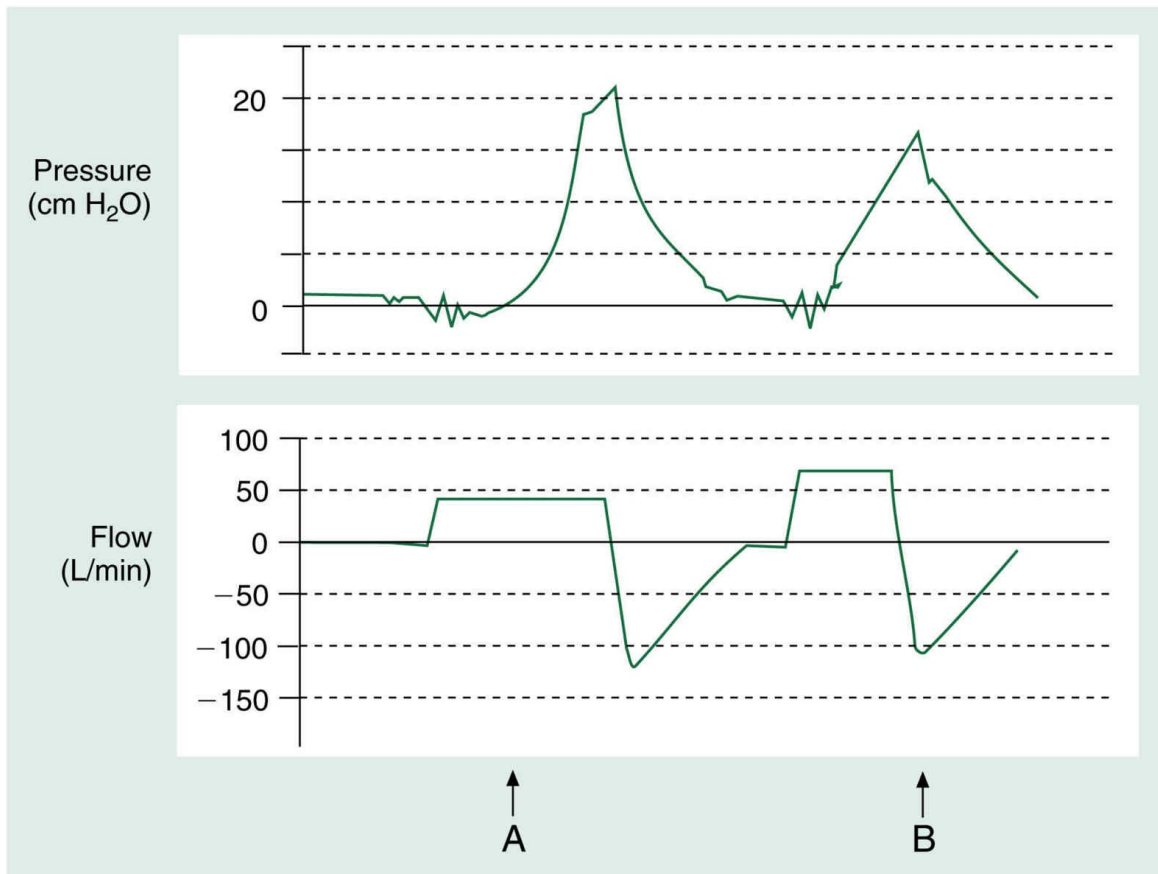
FIG. 5.4 Graphs of volume-controlled continuous mandatory ventilation showing a constant flow waveform. (A) Graphic display indicates that the flow, which is set at 50 L/min, is too low for patient demand. Note the concave appearance of the pressure curve; flow begins at one point, but pressure does not rise with the flow curve until much later. This indicates that the machine is not responding to patient effort. (B) Flow has been increased to 75 L/min. The pressure curve is normal, but sensitivity must also be increased so the flow and pressure curves begin to rise almost simultaneously. In addition, inspiration time is shortened.
