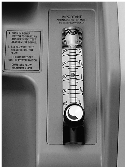
FIGURE 35-3 Close-up view of the low-range flow meter on an oxygen concentrator. (Courtesy AirSep, Buffalo, NY.)
