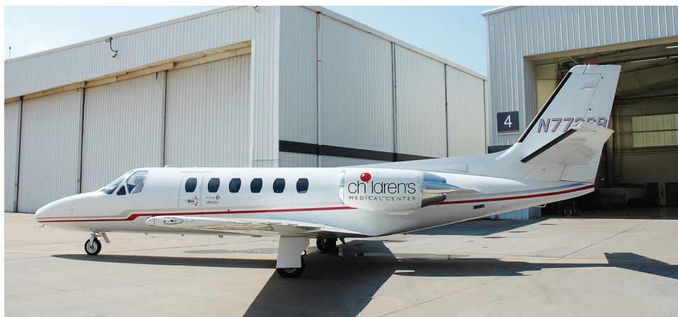
FIGURE 34-3 A jet-engine aircraft that has the ability to transport two patients and five medical crew members within a pressurized cabin. (Courtesy of Children's Medical Center, Dallas.)
