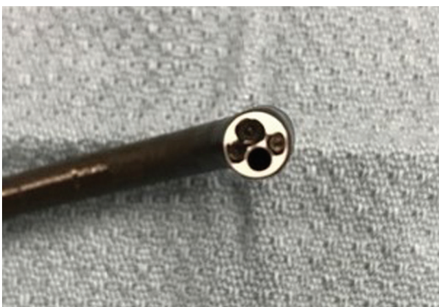
FIGURE 7-4 Distal tip of a 5.0-mm outer diameter bronchoscope with two light bundles, a camera (11 o'clock), and a working and suction port opening (5 o'clock).
