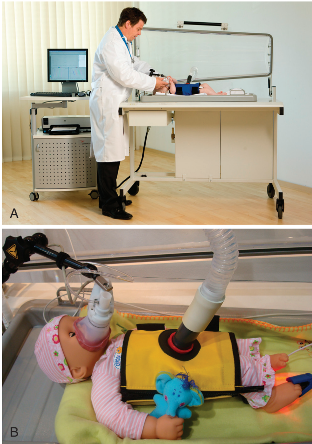
FIGURE 5-1 A , Positioning a patient in a “baby box” plethysmograph. B , Close-up of sedated baby with face mask, putty to form a seal, and pneumatic belt to perform the “hug technique.” (Courtesy CareFusion.)
