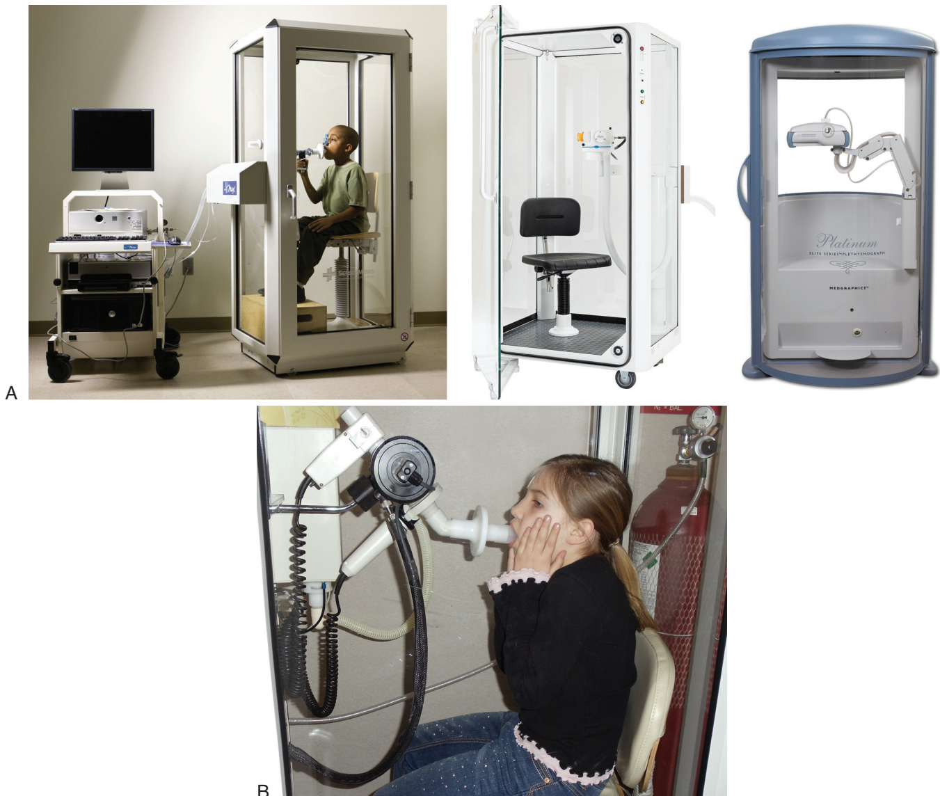
FIGURE 5-12 A, Three different vendor body plethysmographs. (Courtesy CareFusion, nSpire, and MGC Diagnostics.) B, Child supporting cheeks, panting, while performing lung volumes using a body box. (Courtesy Katrina Hynes.)
