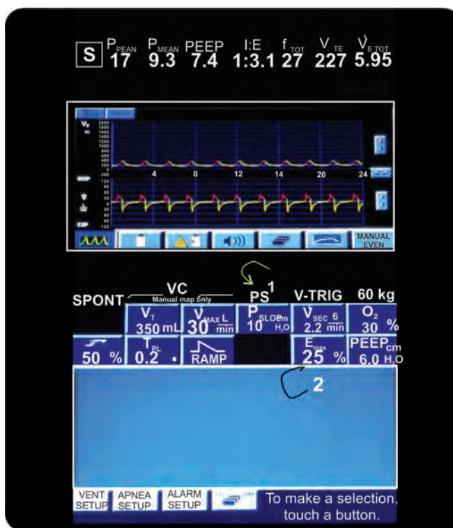
Fig. 5: Ventilator in spontaneous pressure support mode [1—the support pressure during inspiration; 2—expiratory sensitivity: this means when inspiratory flow drops to 25% of the peak value, the ventilator will switch to expiration]
